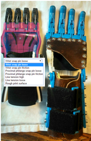
Figure 2: Mockup of common issues in dropdown box and an overlay of the 3D model for the Cyborg Beast to indicate where an issue exists in pink. Photo: [4]
