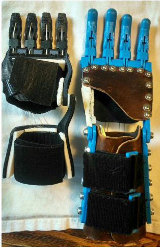
Figure 1: A comparison of Cyborg Beast (left) to Talon 2.0 (right) posted to e-NABLE Google+ community. Photo: [4]
