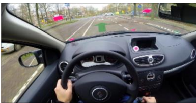
Figure 1: The navigation directions are projected on a HUD mapped directly to road and the horizon from the perspective of the driver.
