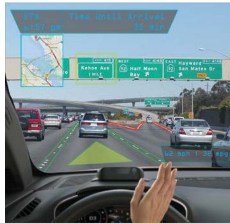
Figure 3. The Transit display highlights the current location along the route to a destination, as well as estimated time to arrival (ETA), speed and fuel economy.
