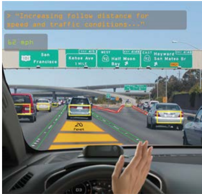
Figure 1. The Defensive Driving display highlights known obstacles in the environment and road markings. Auditory displays (shown in orange quoted text) will give additional information regarding the behavioral intentions of the vehicle.
