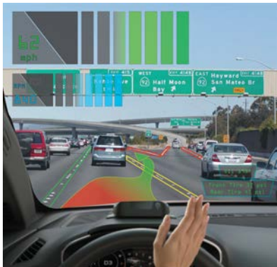
Figure 2. The Thrill-Seeking display emphasizes the speedometer and RPM and provides tire pressure information.
