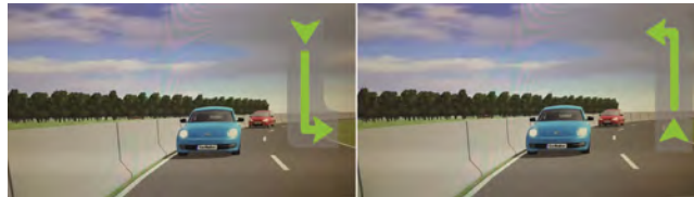
Figure 2: Augmenting upcoming maneuvers when driver-passengers face backwards ( explicit feedback ). The vehicle driving a left turn presents the maneuver symbol in either perceived (left) or logical (right) direction.
