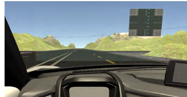
Figure 3: When vehicles pass future intersections with high speed, a map preview from a birds-eye perspective may help users to understand system decisions.
